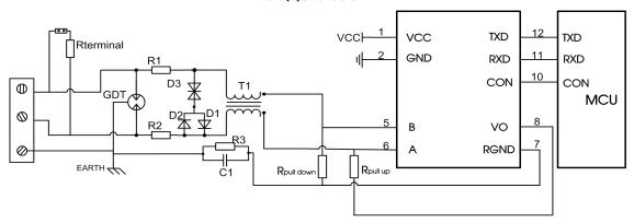
Fig. 2: Recommended protection circuit
